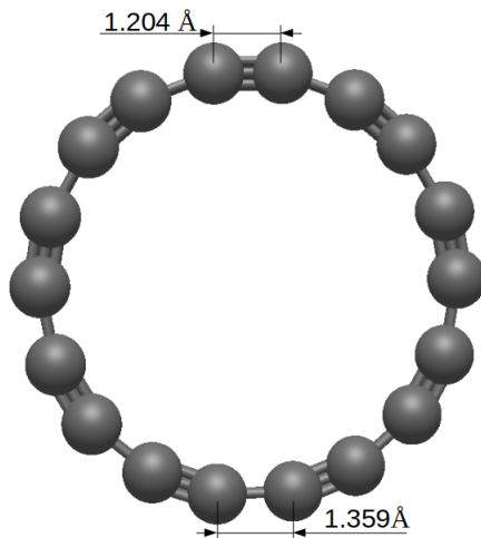
Figure 6.1: Optimized polyynic ( D_{9h} ) structure of C_{18} ring, relaxed using the range-separated hybrid functional HSE [21] based on the GGA-PBE XC functional. A high fraction of HF exchange of a = 0.8 was employed, as suggested by previous studies [292, 313].
